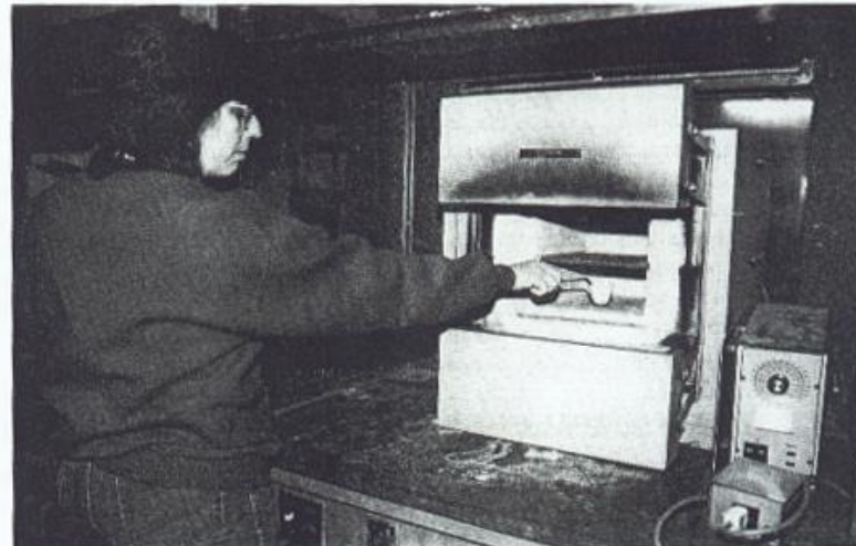
FIGURE 3-8 A muffle furnace used in determination of ash content. (Courtesy of Karen Anschutz, University of Arkansas Animal Nutrition Laboratory, photograph by James Herndon)
