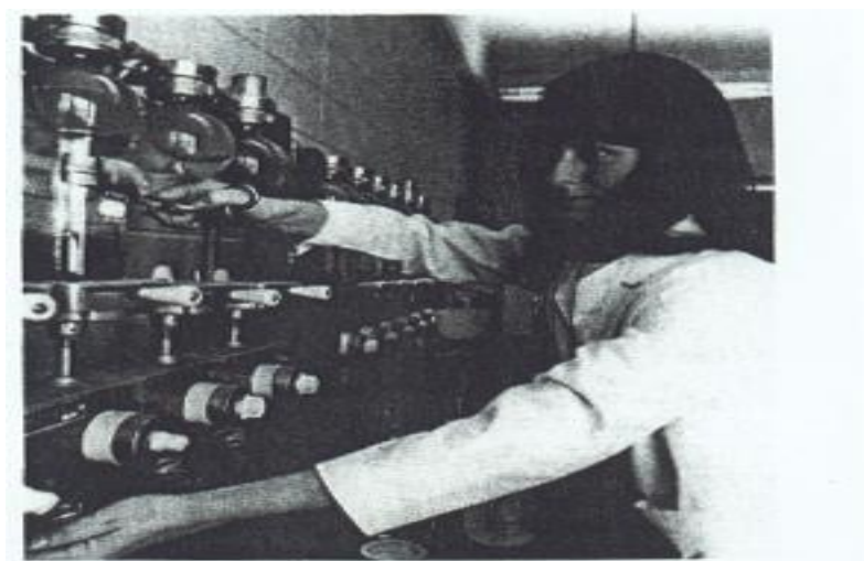
FIGURE 3-7 A feed sample boiled in dilute acid for 30 minutes is being removed for filtering in a crude fiber determination. (Courtesy of the University of Georgia College of Agriculture Experiment Stations)
