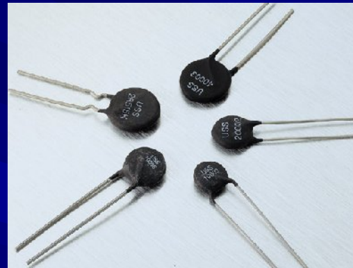
Current limiter thermistor
