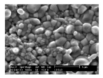
Fig.6 Microstructure of CuFe<sub>2</sub>O<sub>4</sub> based-thick film fired at 1000°C for 1 hr (without glass frit concentration)
