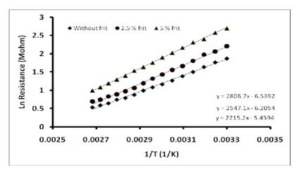
Fig.8. The relation between In Electrical Resistivity and 1/T of CuFe<sub>2</sub>O<sub>4</sub> based-thick film fired at 1000°C for 1 hr (with : 0; 2,5, 5% glass frit concentration)
