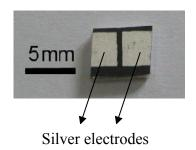
Fig.2. A typical thick film thermistor.
