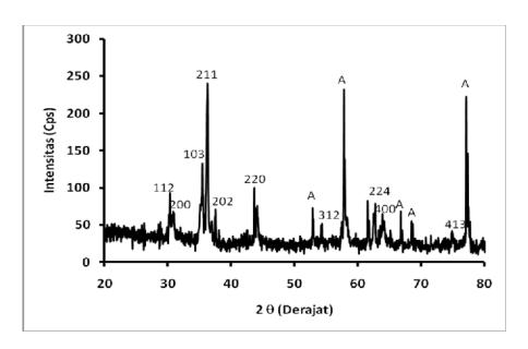
Fig.3. XRD profile of CuFe<sub>2</sub>O<sub>4</sub> based-thick film fired at 1000°C for 1 hr (without glass frit concentration)
