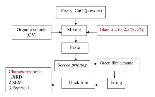
Fig.1. Flow diagram of the experiment procedure.
