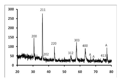
Fig.5. XRD profile of CuFe<sub>2</sub>O<sub>4</sub> based-thick film fired at 1000°C for 1 hr (with 5,0 % glass frit concentration)
