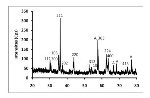
Fig.4 XRD profile of  $CuFe_2O_4$  based-thick film fired at 1000°C for 1 hr (with 2,5 % glass frit concentration)
