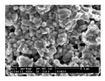
Fig.7 Microstructure of CuFe<sub>2</sub>O<sub>4</sub> based-thick film fired at 1000°C for 1 hr (with 2,5 % glass frit concentration)
