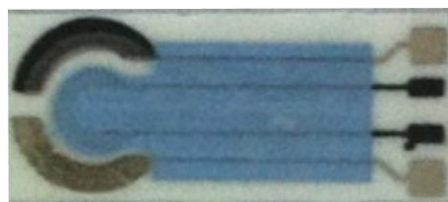
Figure 3. Final device structure after formation of KCl layer over Ag/AgCl reference electrode.
