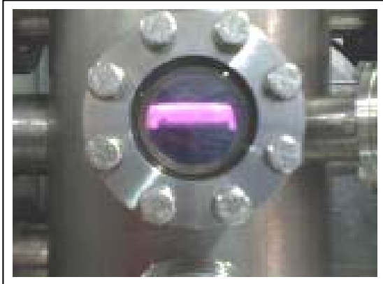
Figure 1: Plasma in the reaction chamber of PECVD system, during the growth process.
