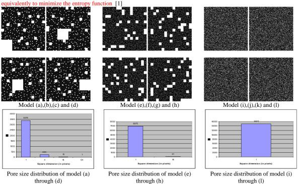
Figure 1. Twelve models of Random Sierspinski Carpets with their associated pore size distribution.
