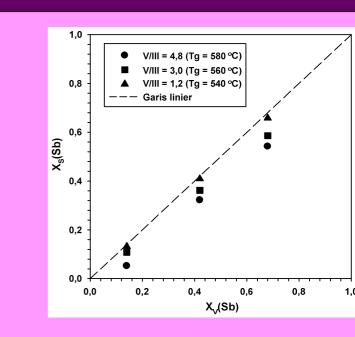
Fig. 1. Sb distribution coefficient for GaAs1-xSbx layers grown on GaAs substrate
