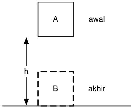
$$\begin{aligned} W \text{ gravitasi} &= \int_A^B \vec{F}_{\text{grav}} \cdot d\vec{l} \\ &= \int_A^B m \cdot g (-\hat{k}) \cdot (dx\hat{i} + dy\hat{j} + dz\hat{k}) \\ &= -m \cdot g \int_A^B dz \\ &= -mg (z_B - z_A) \\ &= -mg (-h) \\ &= mgh \end{aligned}$$
