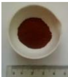
Figure 1. Visual appearance of Fe 2 O 3 powder prepared using precipitation method.
