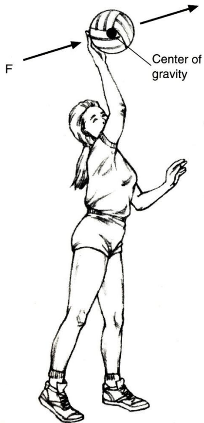
Fig. 4.18. No spin is imparted to a volleyball when force is directed through its center of gravity. Reprinted from Luttgens et al. 1992.
