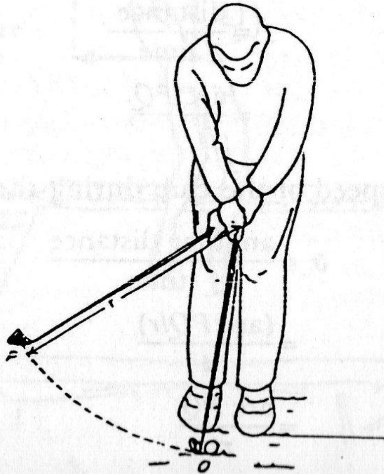
Figure 4-6. The velocity of the club head is equal to the product of its angular velocity and the radius of rotation.
