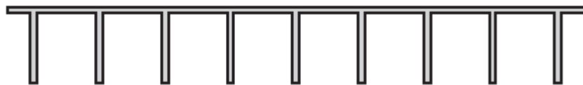
is analogous to a One-Way Pan Joist Slab (easier to build, accessible voids, lower structural performance)
