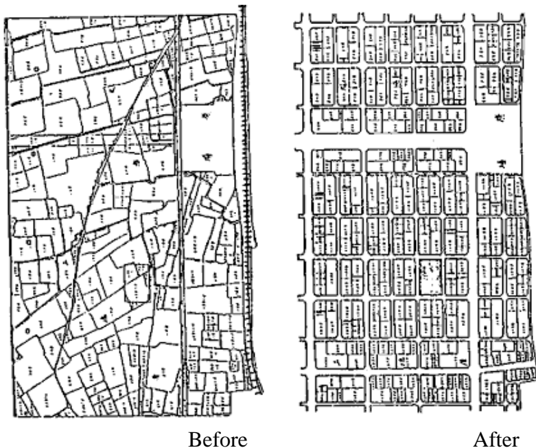
Picture 1 Example of LC project in Kaohsiung City, Taiwan
