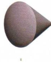
Figure 3.3 – For a solid angle that measures 1 steradian,  $A = r^2$ .
