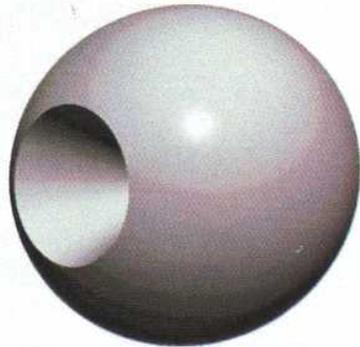
Figure 3.2 – A 1-steradian solid angle removed from a sphere.
