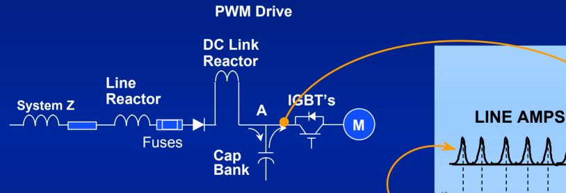
CAPACITOR CAN FILL ONLY WHEN PEAK LINE VOLTS AT A ARE ABOVE CAPACITOR VOLTS: \* LINE AMPS CHARGE CAPS IN VERY UNEVEN BUMPS [NOT SINE WAVE!]
