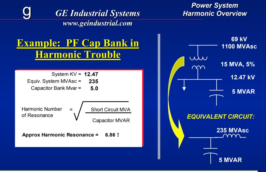
CAP BANK AND SYSTEM Z RESONATE NEAR 7th HARMONIC! ANY DRIVE OR RECTIFIERS ON THE SYSTEM COULD CAUSE HUGE OVERVOLTAGES!
