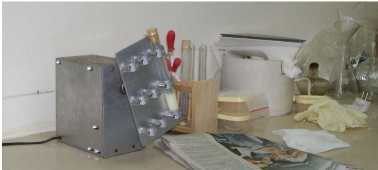
Fig. 1. The process of shaking the solution using a shaking machine.
