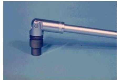
Figure 27 - Point Shoulder Bolt Socket
